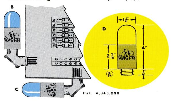
A heavy load hung inadvertently on the installed device could result in damage to the mounting extension. For this reason, side mounting is not recommended without the use of a street ell which facilitates vertical mounting.
