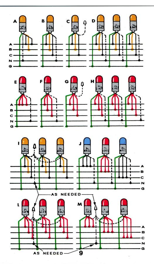
Attach Silent Slaves to the **LOAD** side of Disconnects and to the **LINE** side of Contactors, Relays, Starters, etc.
