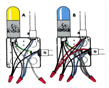
Attach WHITE connecting lead. Remove wire nut or other device from circuit neutral, wrap or twist stripped end of connecting lead around circuit neutral conductors, replace wire nut or other device. If existing circuit contains no neutral conductor, strip end of white connecting lead and cap with suitable wire nut. DO NOT ATTACH WHITE CONNECTING LEAD TO CIRCUIT IF NO NEUTRAL IS PRESENT!
